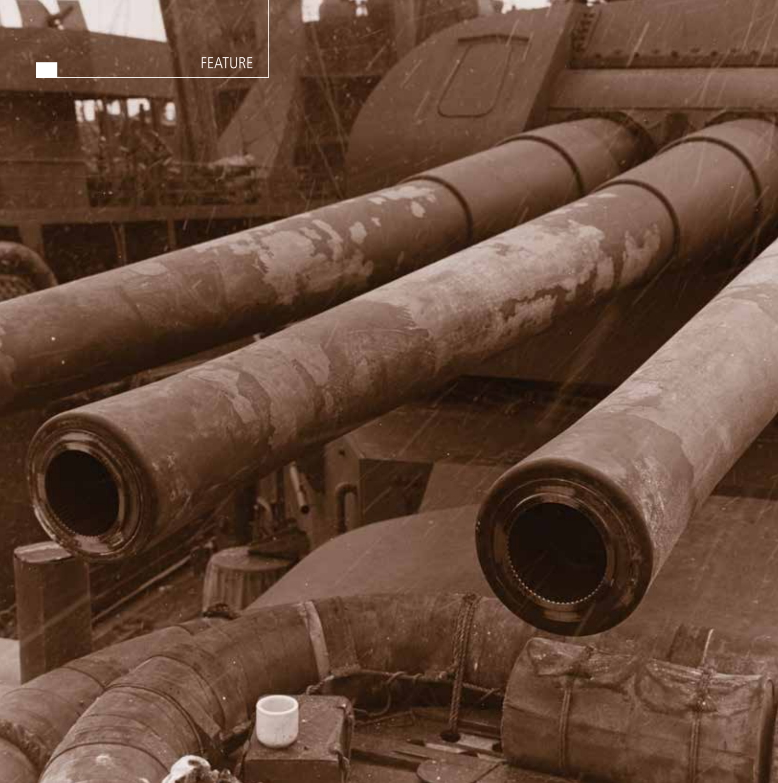
The 8-inch/55-mm guns of Turret 3 on the USS SALT LAKE CITY (CA-25). Notice the heat scale on the tubes from extensive firing during the action at Dutch Harbor in the Aleutian Islands in March of 1943. If you look closely, you can see snow flakes falling. Photo courtesy of the Naval History and Heritage Command.
